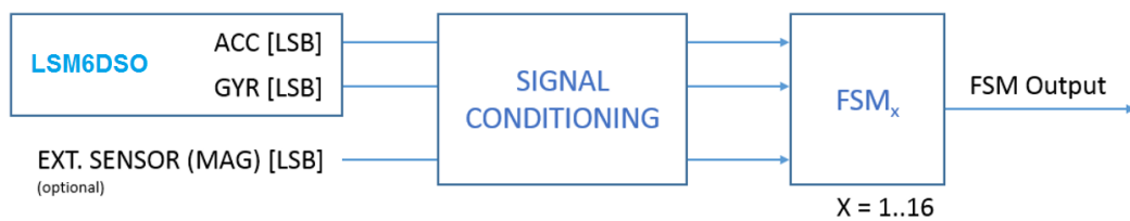
Figure 2. State machine in the LSM6DSO
